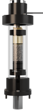
Figure 39: Example of an experimental setup compatible with an instrumented micro-CT scanner, for permeability evaluation.
